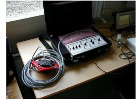
Power amplifier for driving passive hydrophones and underwater loudspeakers.
