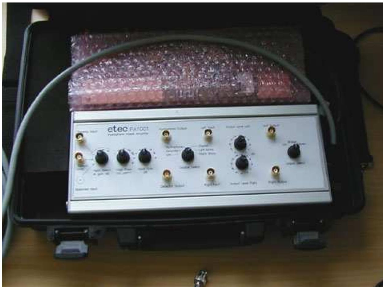
This amplifier is a stand alone unit with a power amplifier and a hydrophone receiver amplifier complete with builtin envelope or "click" detector and batteries and charger supplied all together in a watertight suitcase.
